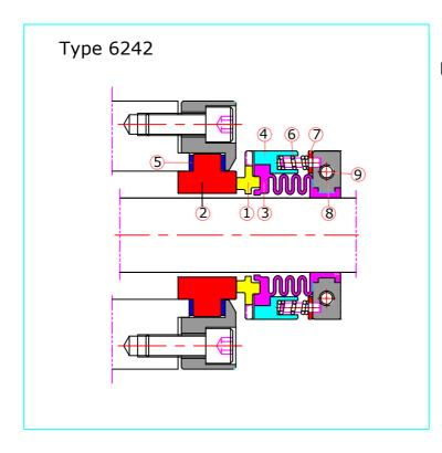
Part No. Description Seal Ring 1 Seat 2 Bellow 3 Spring Holder 4 Gasket 5 Spring 6 7 Thrust plate Clamp Ring 8 Allen Screw 9
